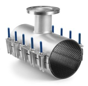
The FST is in fact a reinforced double band clamp with a flanged outlet. The standard working range is 20mm. The upper body is reinforced to accomodate the installation of valves and drilling equipment.
